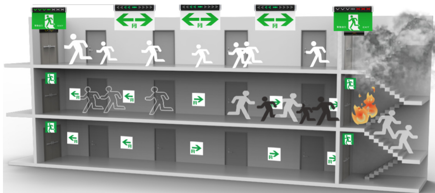
Figure 2. A dynamic escape system for hospital.
