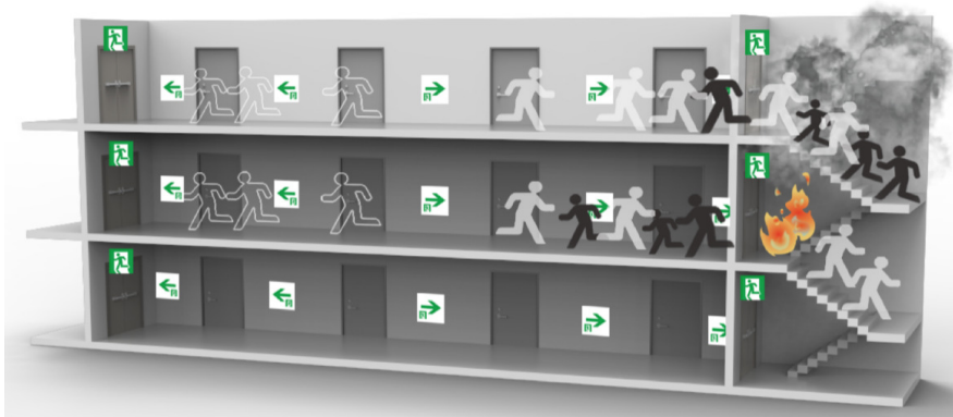
Figure 1. Static escape system for hospital.
